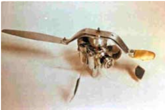
Uncontrolled but stable VTOL machine having acoustic control of height. Vehicle body spins.
