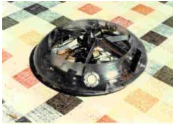
Underside of ducted fan machine showing ultrasonic whistle and microphone.
