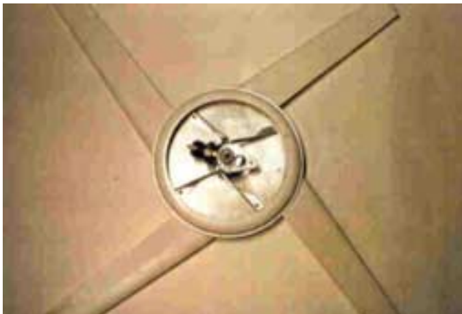
Four blade, cold, tip jet powered machine driven by centrifugal compressor.
