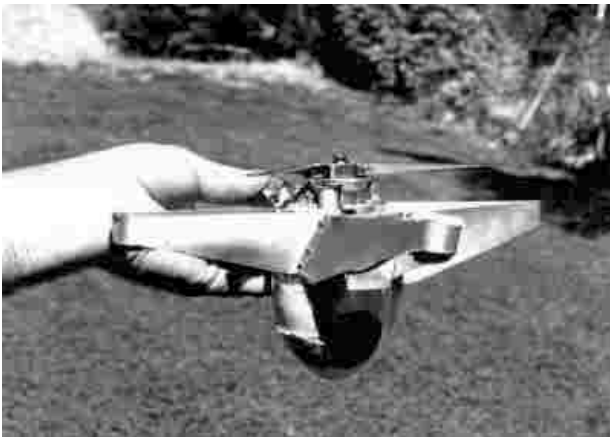
Highly energetic machine using cyclic pitch controlled open blades with counter torque vanes.
