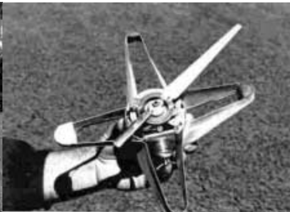
Top view showing single blade cyclic pitch prop.
