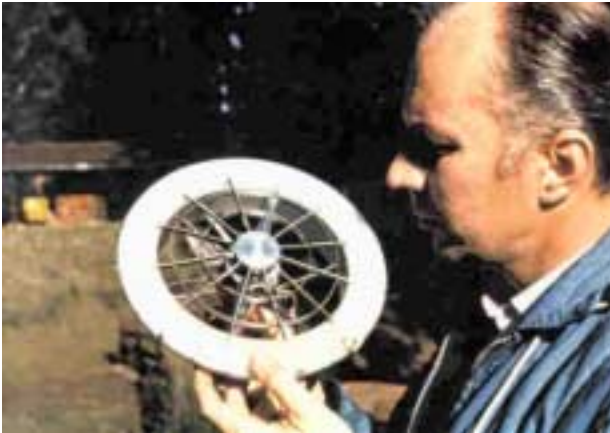
Original ducted fan machine with ultrasonic height control and anti-collision system.
