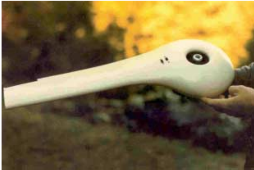
15 pound lift Boomerang with full control for autonomous flight. (A patent was issued to Shoulders for the control system.)
