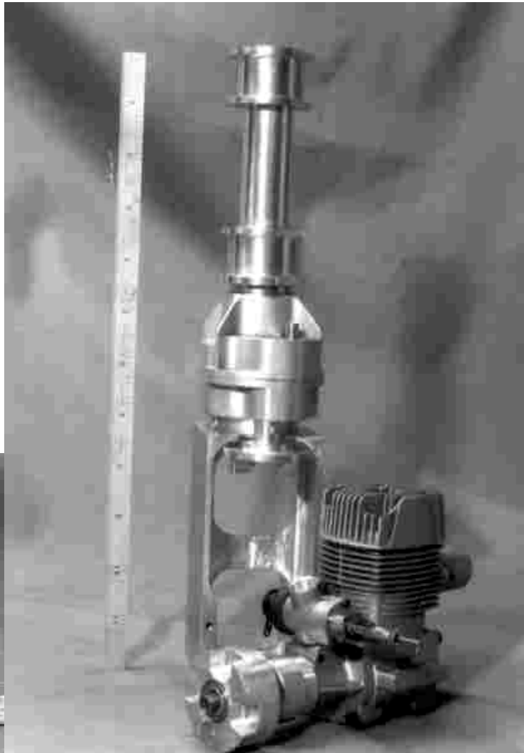
Free piston gas generator developing 2 ghp output.
