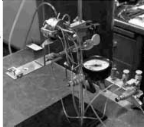
Pressure jet engine using propane fuel. Shown in test cell.
