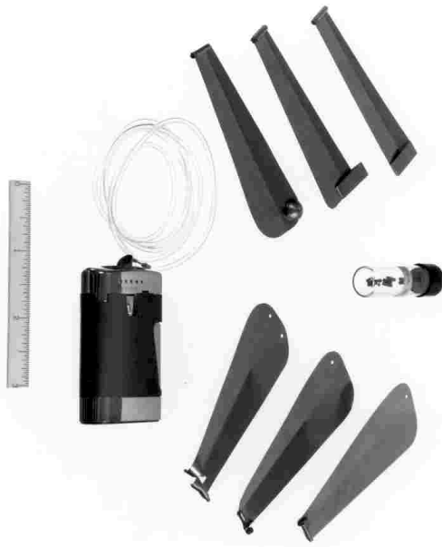
Solid rocket powered, single blade rotors for testing takeoff from unprepared area.
