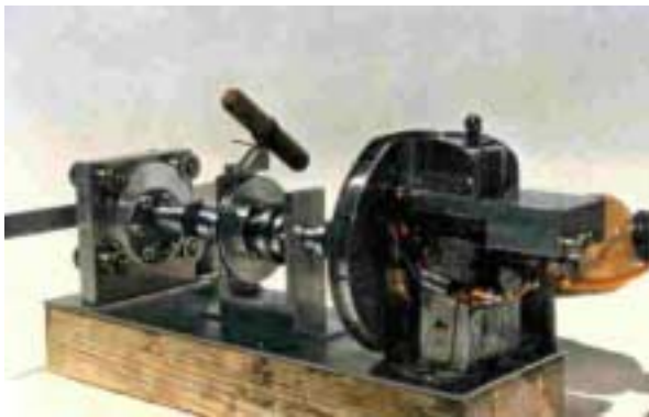
0.15 cu. inch diesel engine shown with hydraulic dynamometer, starter, cooling fan and muffler. Entire assembly is enclosed in sound proof housing to reduce noise level to 35 db at 10 feet.
